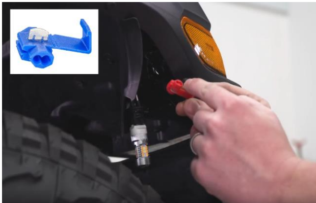
Use a splice snap clip to splice into the white and orange wire.
